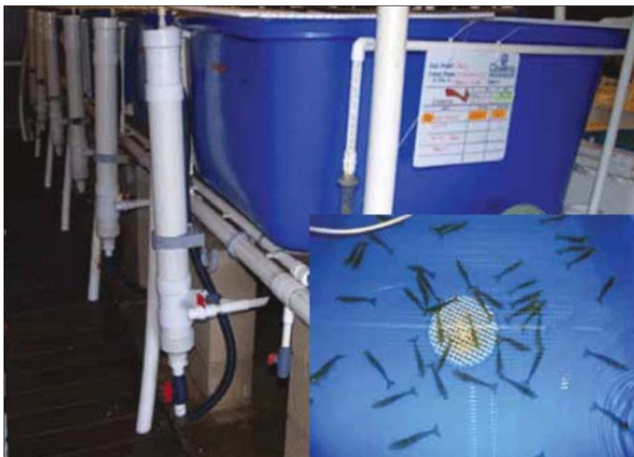
The experiment was conducted in an indoor flow-through water system with a series of 550-L polyethylene tanks.
