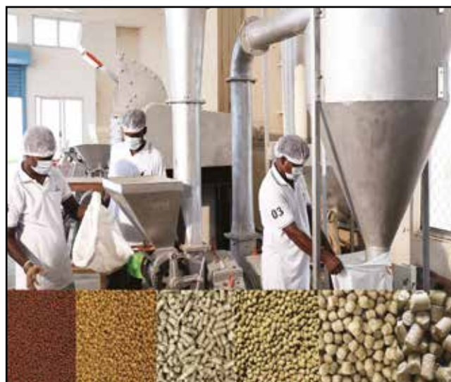
Pilot-scale feed processing infrastructure of CIBA for making formulated pelleted feeds for farmed fishes and shrimp
