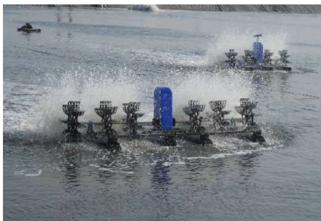
Fig. 5: Positioning of aerators is very important to accumulate sludge at center of the pond
