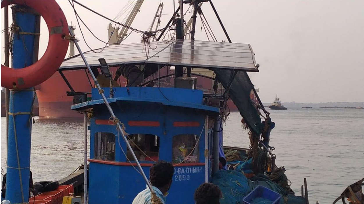
Solar panel installed on the roof of Deck
