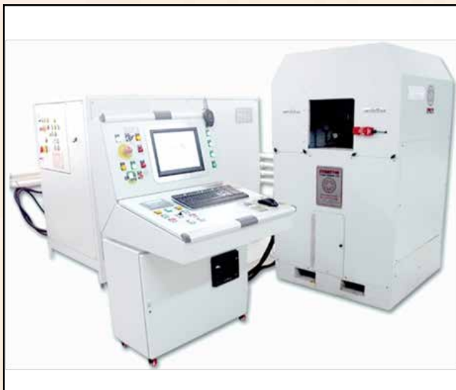
High pressure processing equipment (Photo Courtesy: ICAR-CIFT, Kochi)
